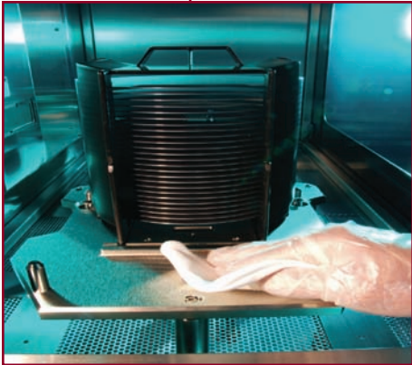
Figure 5 – Maintaining cleanliness of wafer loading area is critical
