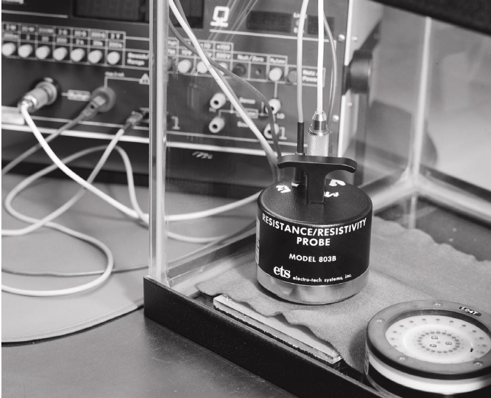
Figure 1. Surface resistivity of a fabric being measured in a controlled humidity chamber.
