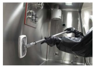
Figure 1. Isolator cleaning tool in use
